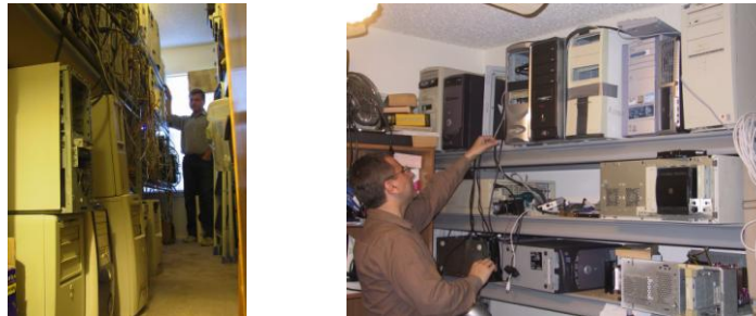
Figure 30. The test grid, side by side there are around half of a hundred CPU blocks connected via network switches.
